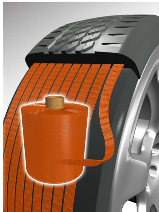
Milliken Cap Ply tape is applied directly onto the tyre
